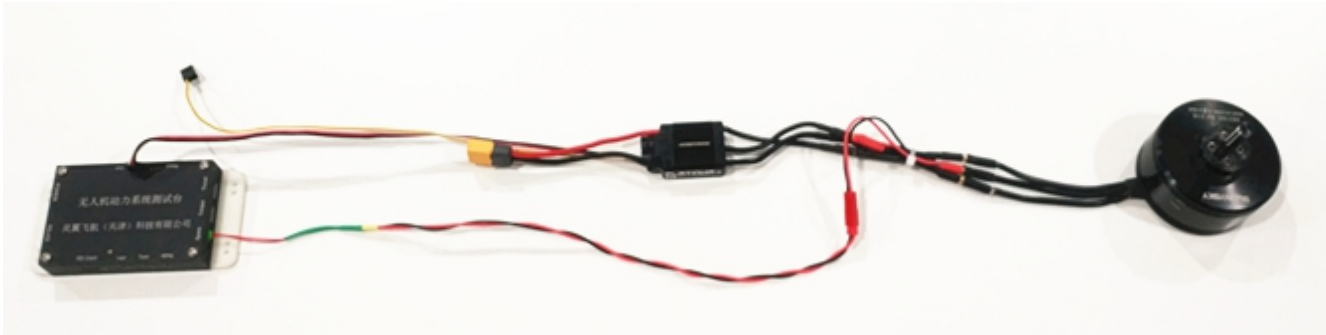
Fig.2.2 Signal Cables Connection
