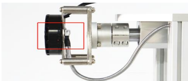
Fig. 2.3.1 Installation of Temperature Probe
