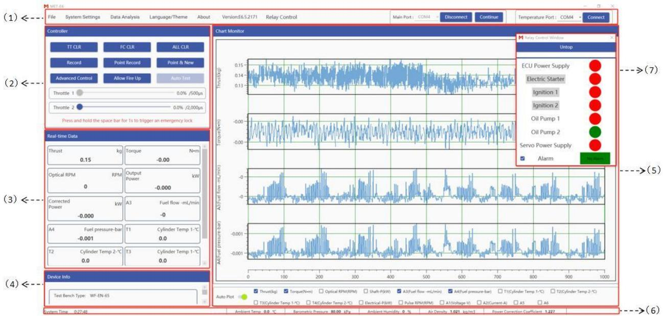
FIG 6-1 Main Interface of the software
