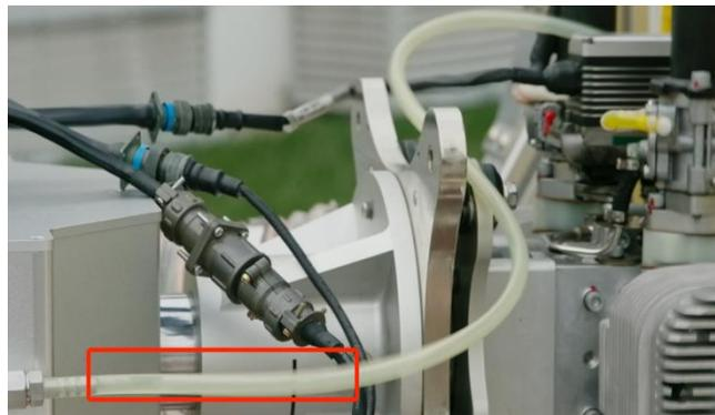
FIG 8-3-2 Engine oil absorption
