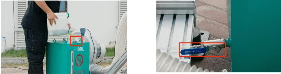
FIG 8-3-1 Fill the fuel tank and open the fuel tank switch
