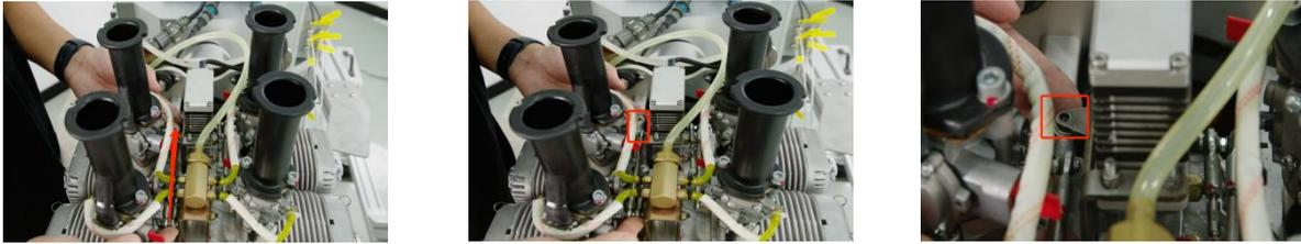
FIG 4-8-1 Adjust the servo rocker arm position to align with the tie rod mounting hole.
