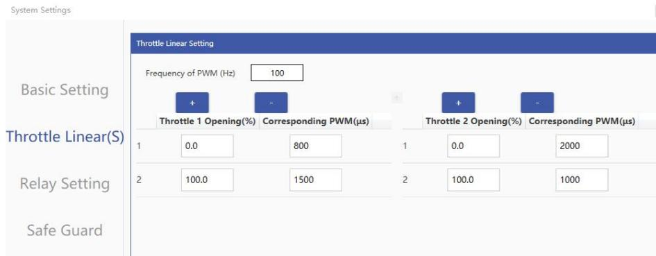
FIG 7-1-2 The throttle linearity setting
