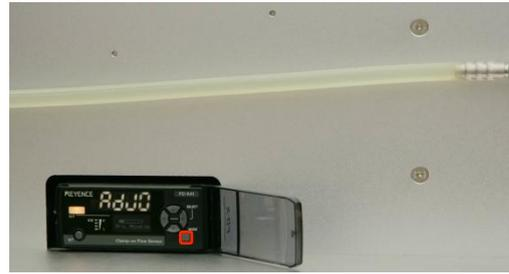
FIG 8-3-6 Press the "MODE" key to complete it.
