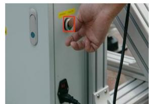
FIG 8-4-1 Close the fuel tank outlet and turn off the power switch
