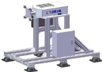
FIG 3-1-1 WF-EN-55 engine test bench
